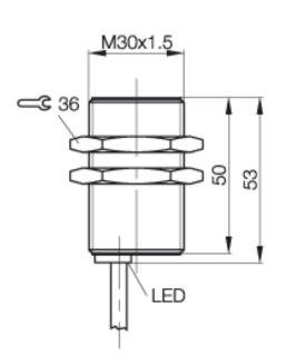
Inductive Sensors BES M30MI-POC15B-BP02 M30x1.5 x 53 normally-closed Sn=15mm shielded
